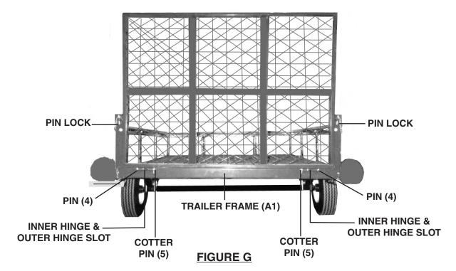
22. Raise the Rear Ramp (A5) to its up position. Then, lock the Rear Ramp in place with the two Pin Locks. (See Figure G.)
